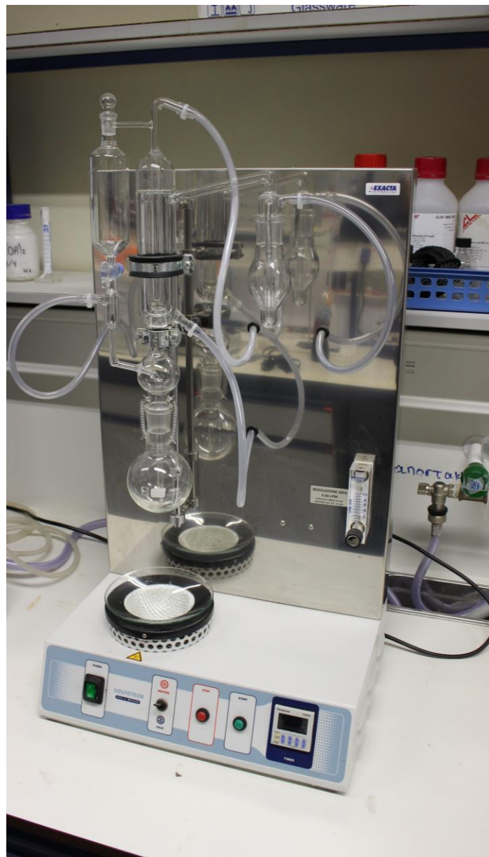
Exacta Solfotech S apparatus for the determination of Sulphur Dioxide according to the official method OIV-AS-323-04
