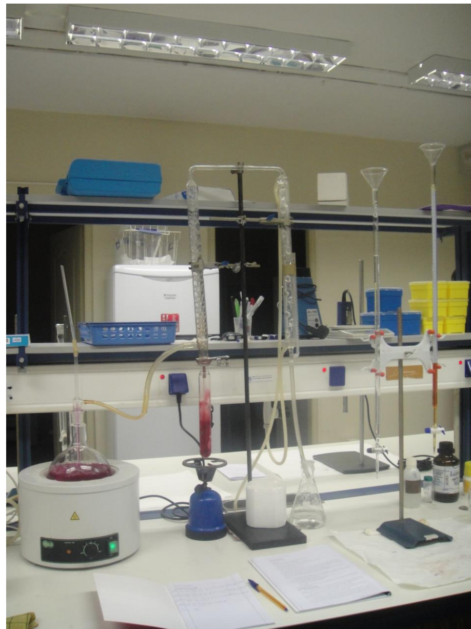
Steam distillation apparatus for the determination of Volatile Acidity according to the official method OIV-MA-AS313-02
