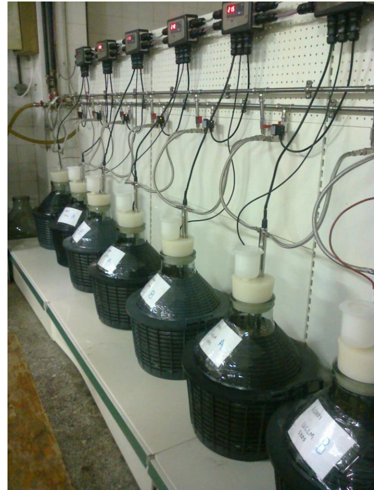
System of micro-vinificators with refrigeration system and solenoid valves
