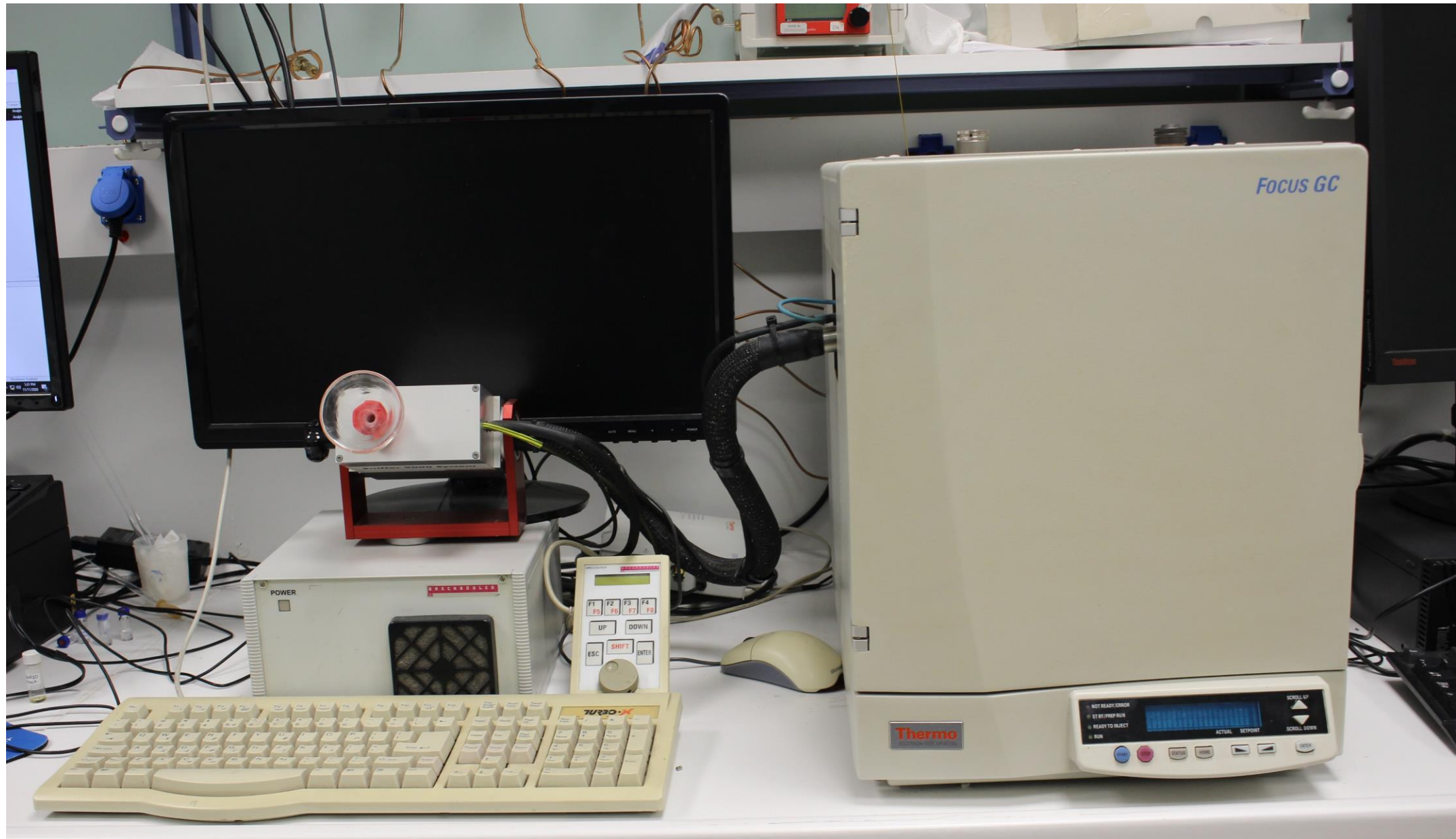
Gas Chromatography system Thermo Focus GC with FID detector and Olfactometer (GC-O)
